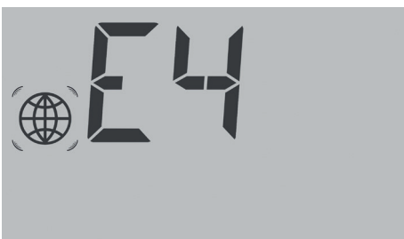
Fig.: Example for a blinking code sequence for Internet - Fault 4
