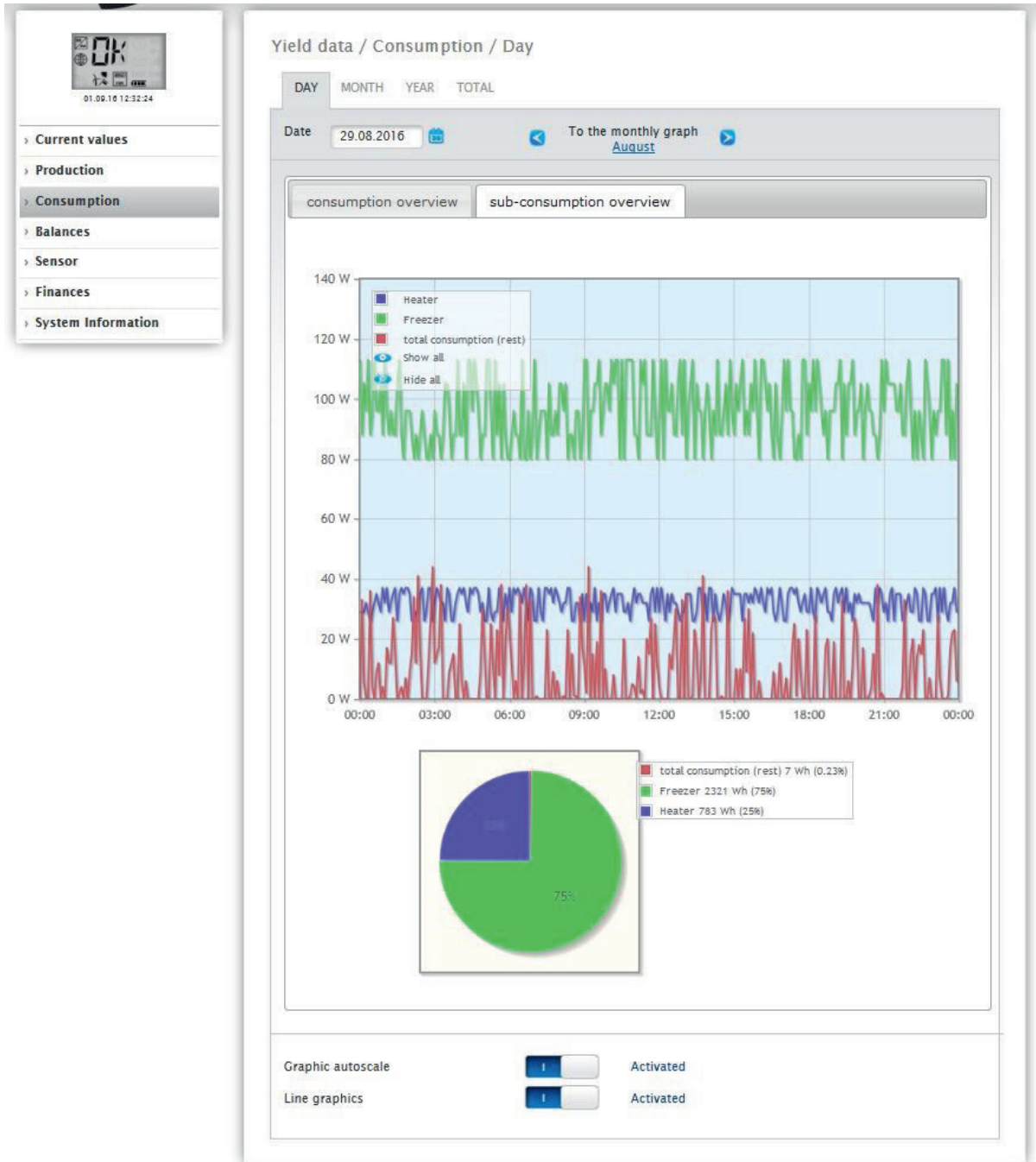
Fig.: Graph of daily consumption with connected appliances and active line graphics in the sub-consumer view
